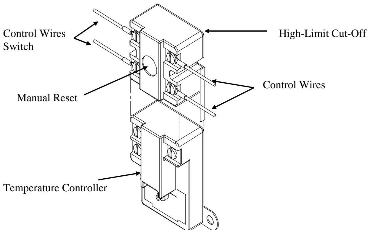
4. Disconnect the high-limit cut-off switch from the temperature controller by pulling the cut-off switch up and away from temperature controller.
