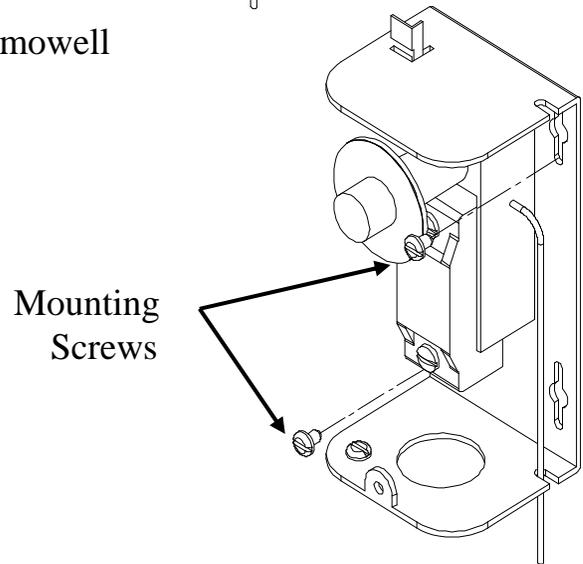
7. Remove control and install new high limit switch by performing above steps in reverse order. (Note: Be sure to place capillary tube into slot in base prior to installing cover.)
