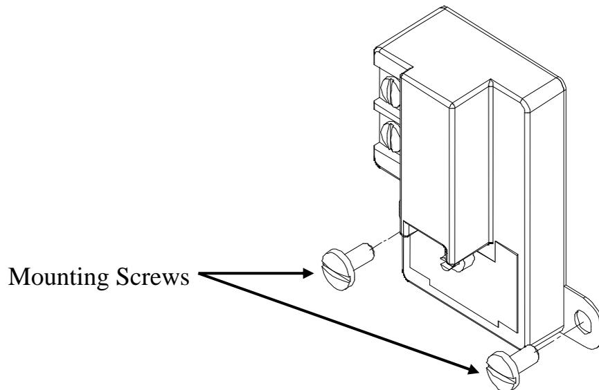
Replace thermostat using the reverse procedure.
