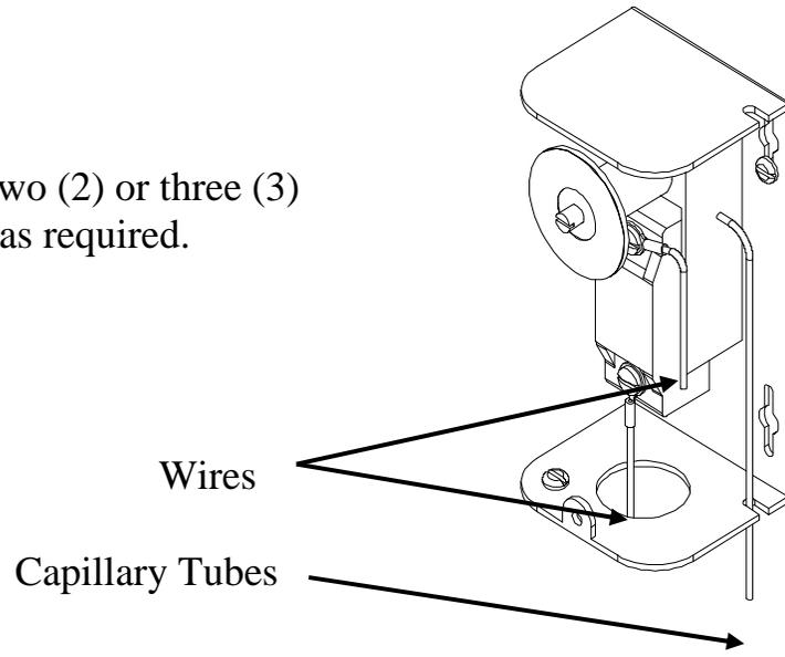
5. Remove capillary tube and bulb from thermowell.
