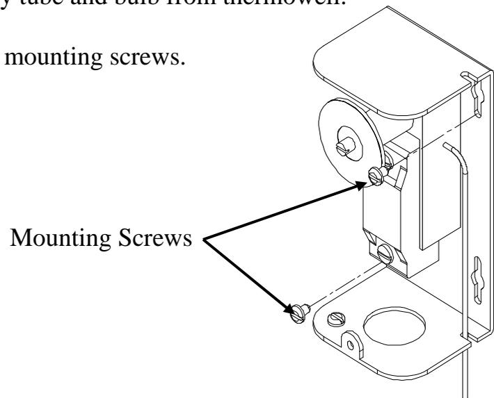
7. Replace thermostat using reverse procedure. (Note: Be sure to place capillary tube into slot in base prior to installing cover.)
